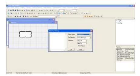
6. Add a static bitmap. Open a blank page (step 3), then on the toolbar, click . Double-click the blank page to display the **Static Bitmap Setting** dialog box where you can choose the bitmap.
